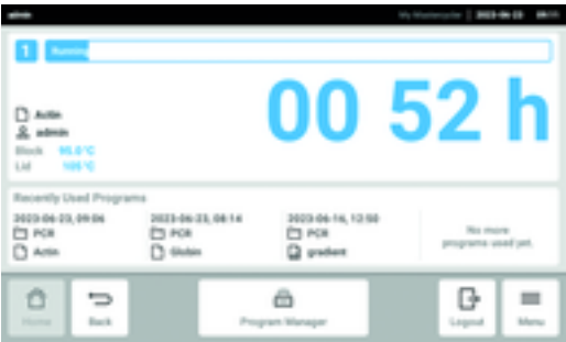
Fig. 3-2: Home screen during execution of a PCR program
